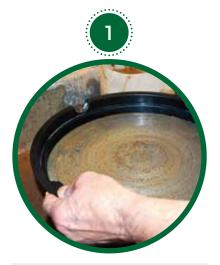
Place BATretainer ring on wheel head at an angle pivot on drive stops
