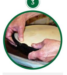
Hold BAT above the BATretainer ring and align correctly before pressing down in place.
